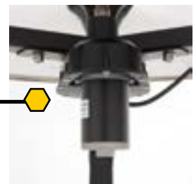
Bottom-mounted motor on a crossbar
